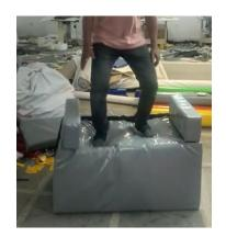
Impact tests have been conducted with people jumping on and falling (thrown) on the furniture. The furniture dissipates the impact and returns to its original shape.
